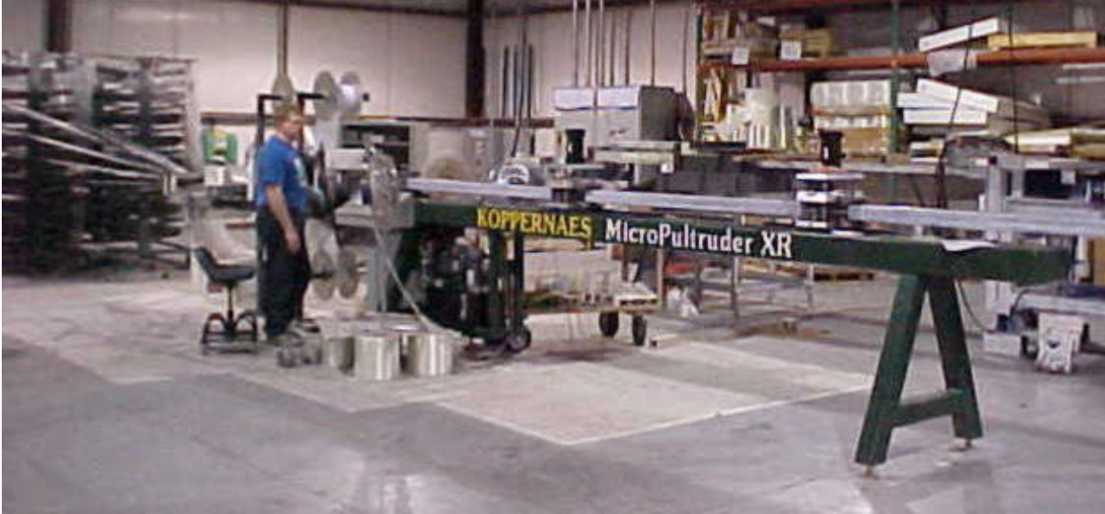
Figure 3 - Pultrusion Process for Carbon Tube
