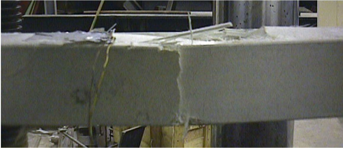
Figure 9 - Photograph of Single Tube Failure
