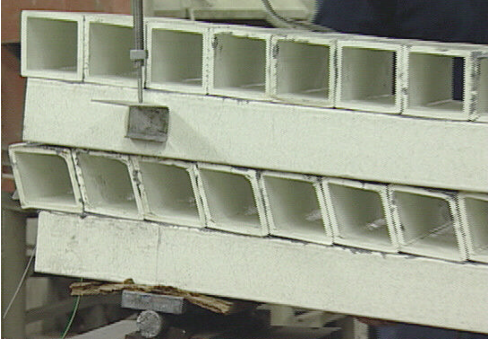
Figure 11 - Photograph of Four Layer Failure
